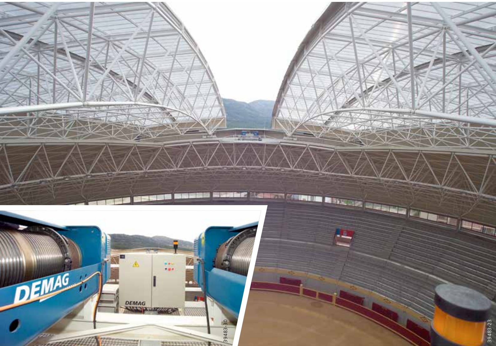
Stationary DH rope hoists used for moving a domed retractable roof
