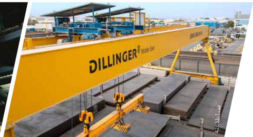
DH hoist in a foundry for safely handling molten masses Full-portal crane with DH hoist units in tandem mode
