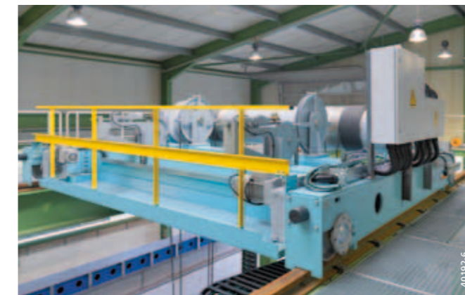
Fully pre-assembled MPW crab with a telescoping gripper for handling tools
