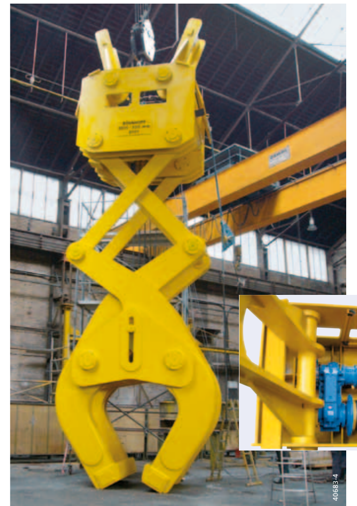
MPW open winch unit employed in a gripper system for transporting steel slabs
