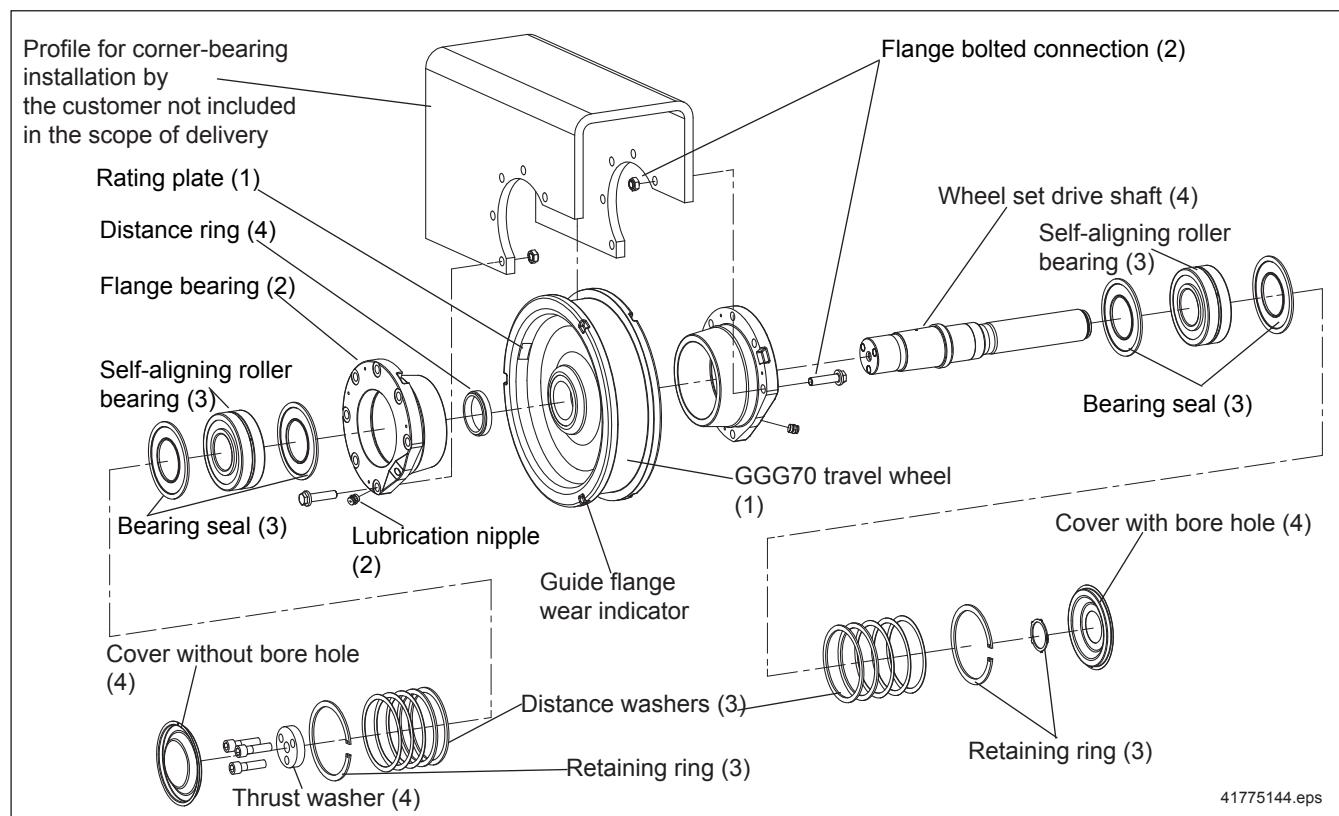
The wheel set consists of four sub-assemblies:
