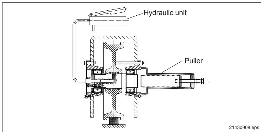
**Disassembly:** A puller is also required in addition to the pump.
