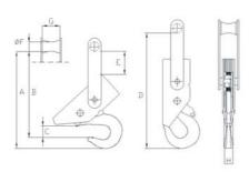
The Automatic Hook is available in 6 sizes from 2 to 20 tons. It is easy to operate, has rugged design and a high reliability.
