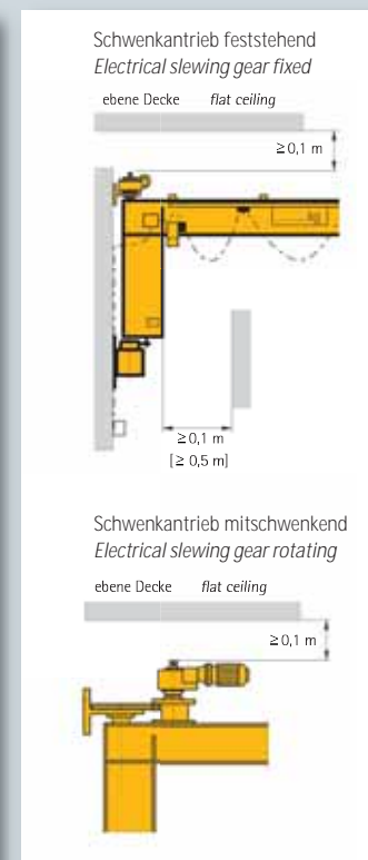
Wandschwenkkrane Wall-mounted slewing jib cranes
