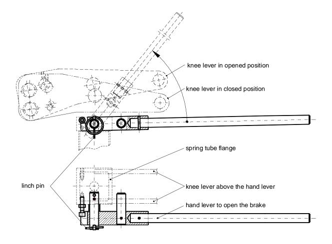
The hand lever is used to open the brake manually in case of an emergency or to service the brake unit. A linch pin secures the hand lever and spacer. The spacer should be permanently attached to the bolt. Remove the linch pin by pulling the spring tensioned ring up and pull the pin out. Slip the hole of the hand lever over the bolt, insert the linch pin in the bolt hole and secure it by pushing the ring down.
