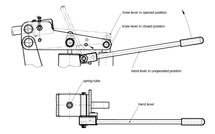
The hand lever is used to open the brake manually in case of an emergency or to service the brake unit. A swivelling device is permanently mounted to the spring tube. For the manual brake opening, the hand lever is to be pushed into the matching hole of the swivelling device.
